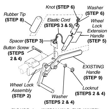
FIGURE 1 - INSTALLING THE WHEEL LOCK EXTENSION HANDLE
